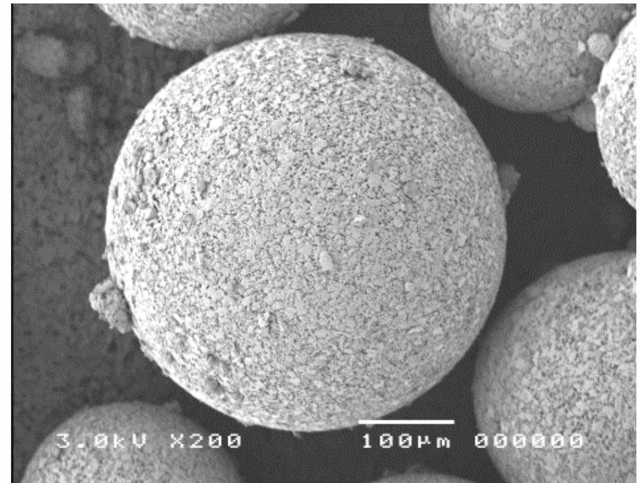
Free-flowing granules with a wide granule size distribution (50–500 µm). Lower granule and tap density vs spray-dried granules.
