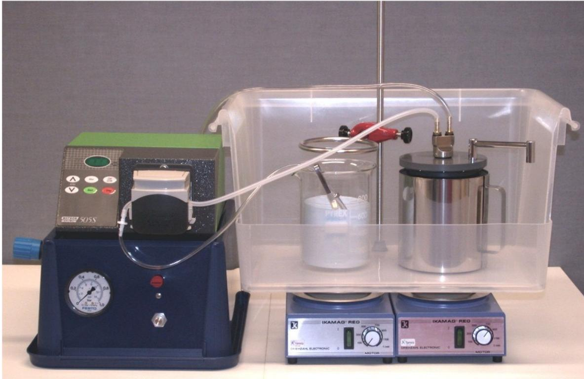
Capacity to granulate up to 6 l powder suspension per hour
