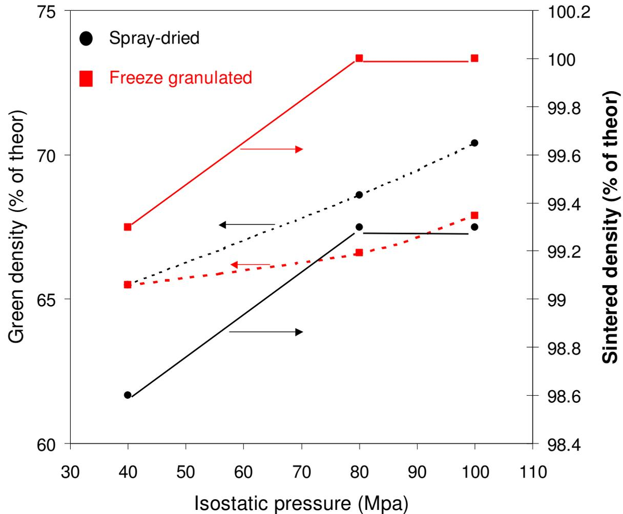
FG requires lower CIP pressure and gives higher sintered density from the same pressed density than SPD does
